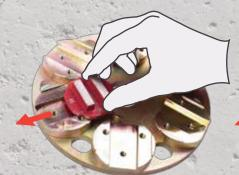
**Installing** diamond tool in **horizontal** angle
