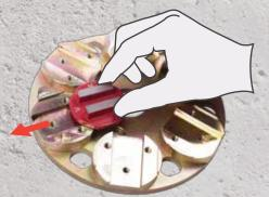
**Installing** diamond tool in **vertical** angle
