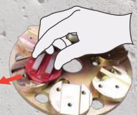
**Installing** diamond tool in **slant** angle
