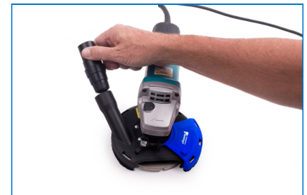
9. Attach the hose adapter. Attach the vacuum hose to the adapter.
