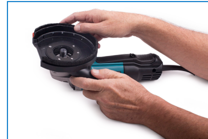
2. Loosen shroud clamp and push shroud on grinder.
