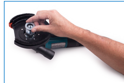
5. If necessary place large washer(s) on cup adapter nut, so cup wheel extends 1/16" - 1/8" beyond shroud.
