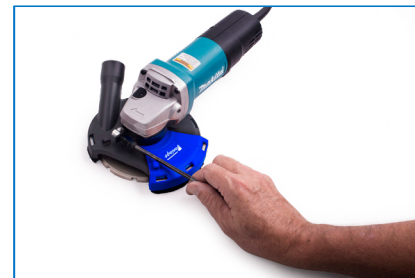
8. Tighten clamp snugly so shroud is secure to grinder. Make sure cup wheel is not in contact with shroud and extends.
