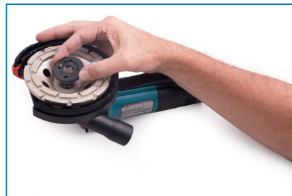
7. Screw hex nut onto cup adapter.
