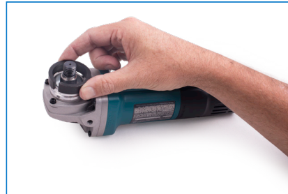
1. You may need to install bushing, so the shroud will fit tightly.
