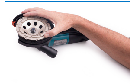
6. Place cup wheel on the adapter nut.
